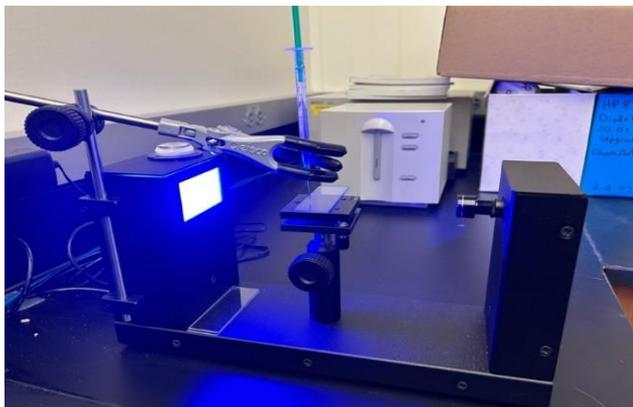
Figure 2. Ossila contact angle goniometer set up.
