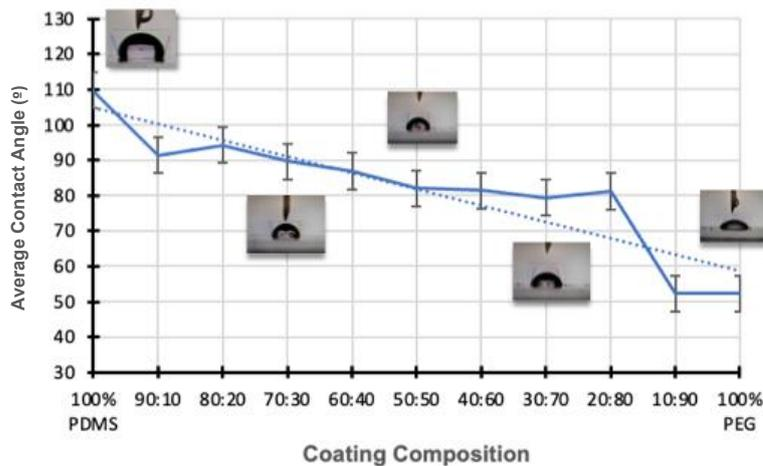
**Figure 8. Graph of contact angle averages of 100:0-0:100 PDMS-PEG ratio blends.**
