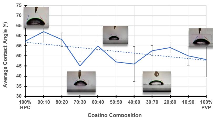
Figure 9. Graph of contact angle averages of 100:0-0:100 HPC-PVP ratio blends.
